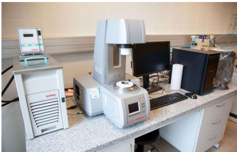
Figure 3.1 Anton Paar MCR 302/ Peltier temperature control (middle), UV curing system (left) and computer (right)
