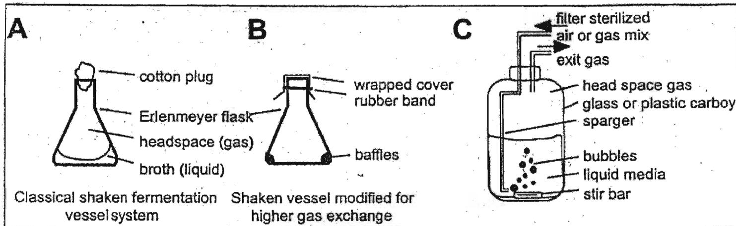
Figure 1.2. Diagrams illustrating common small-scale liquid fermentation systems (Hilton, 1999).
