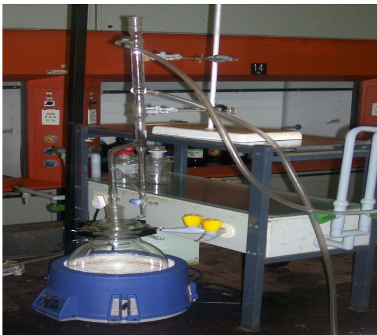
Figure 3.3 Clevenger apparatus for hydrodistillation of aromatic plants
