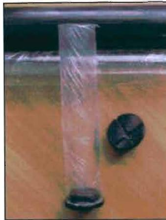
**Plate 4-4: The materials for the capsule comprising of perspex tubing and HDPE end plugs.**
