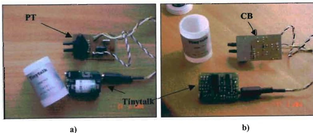
**Plate 4-3: Different views of the Tynytalk data logger and the pressure transducer mounted on a circuit board along with the microprocessor, are shown in a) and b).**
