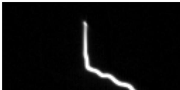
Figure 35 - The bent path a streamer takes for a gap length of 15 cm when approaching the cathode.
