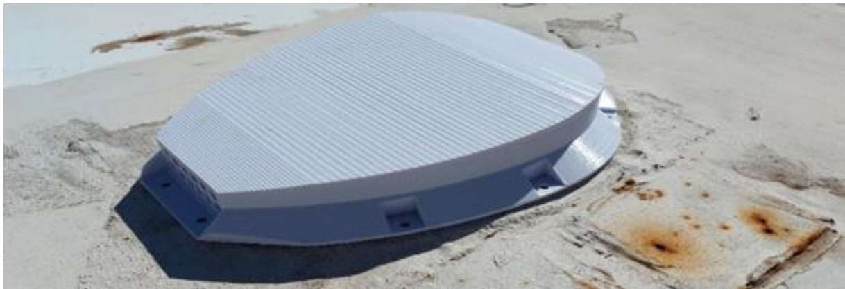
Figure 5 - 25 Side View of the 3D Printed Roof Scoop with the Stair-Stepping Artifact [134]
