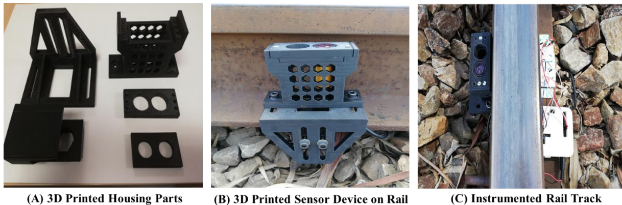
Figure 3 - 5 Custom 3D Printed Wheel Lateral Displacement Measuring Device for Calibrating Wayside Lubricators [10]
