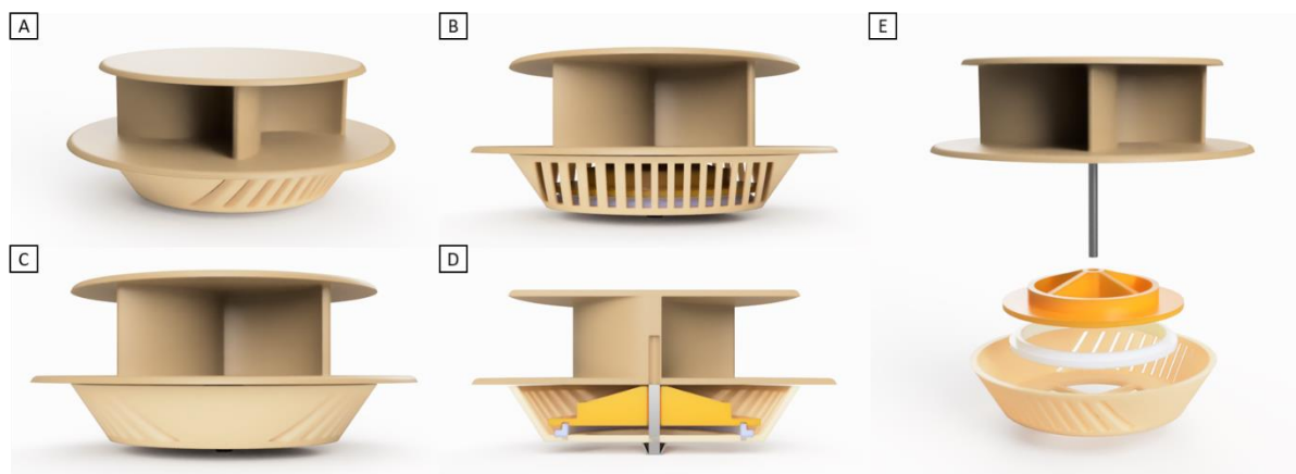
Figure 5 - 7 Concept 2 Isometric View (A), Front View (B), Right View (C), Cross-Section View (D), Exploded View (E)
