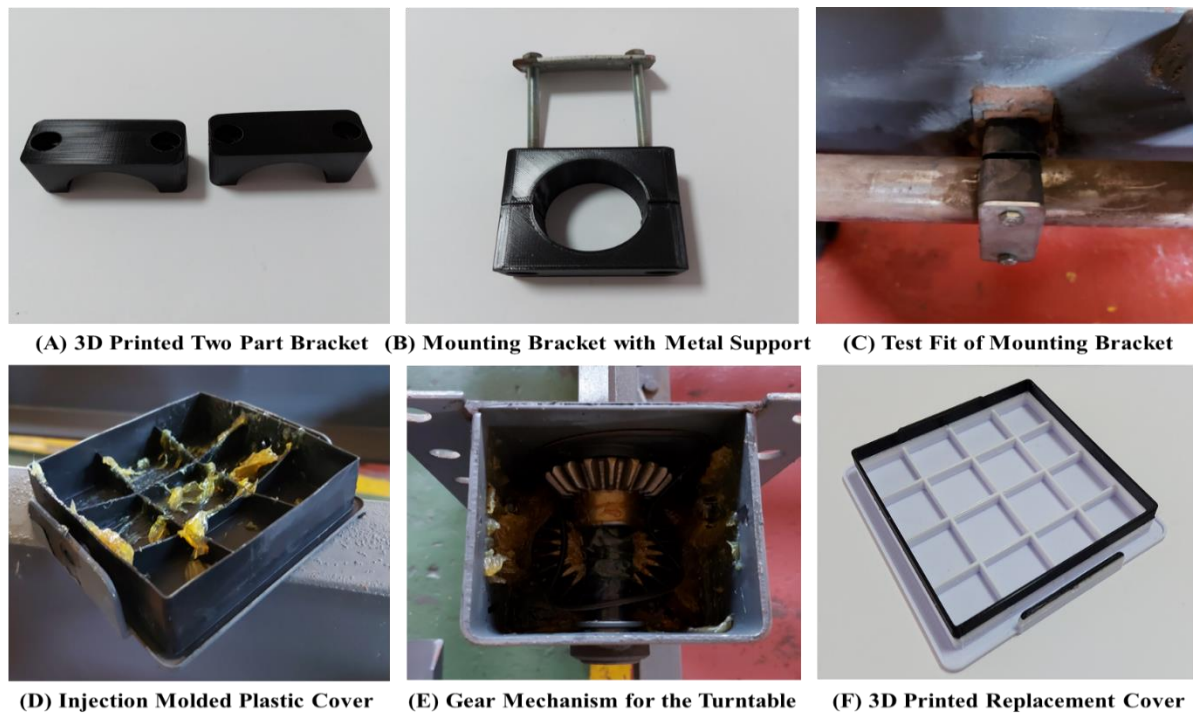
Figure 3 - 6 3D Printed Mounting Brackets and Injection Moulded Plastic Cover [10]
