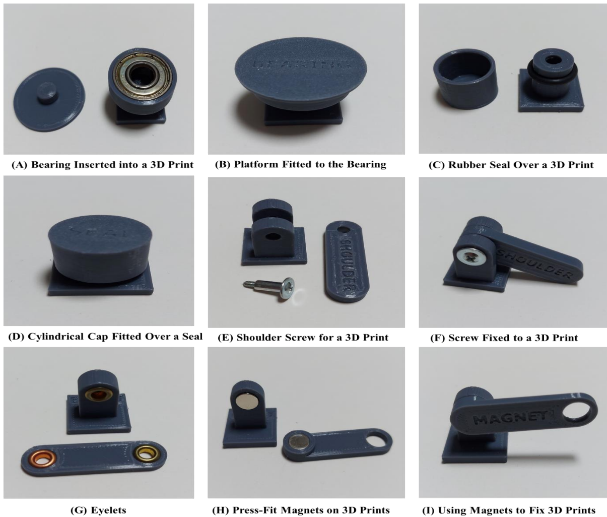
Figure E - 17 3D Printed Parts that Integrate with Bearings, Rubber Seals, Magnets, Shoulder Screws and Eyelets
