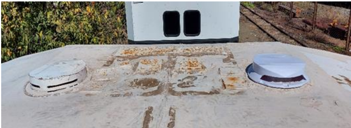
Figure 5 - 27 The Functional 3D Printed Roof Scoop Air Vent Installed [134]
