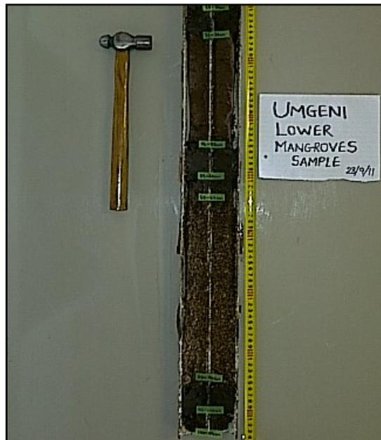
**Figure 32: Green strips to mark the sediment layers/units of the core sample, based on texture and colour.**
