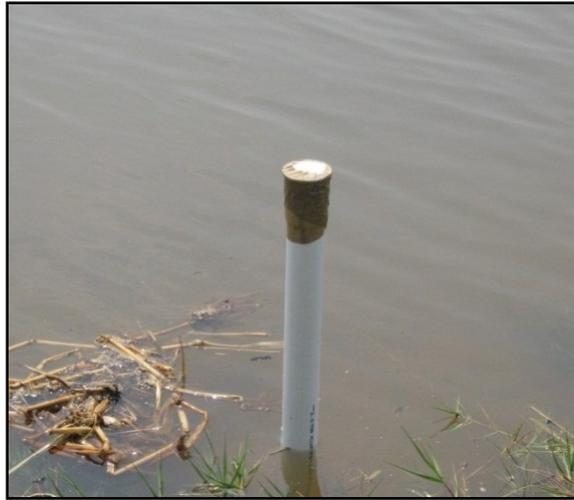
**Figure 30: The placement of the 2 m PVC pipe into the estuarine sediments with the custom made cap sealed at the top to create suction within the pipe.**
