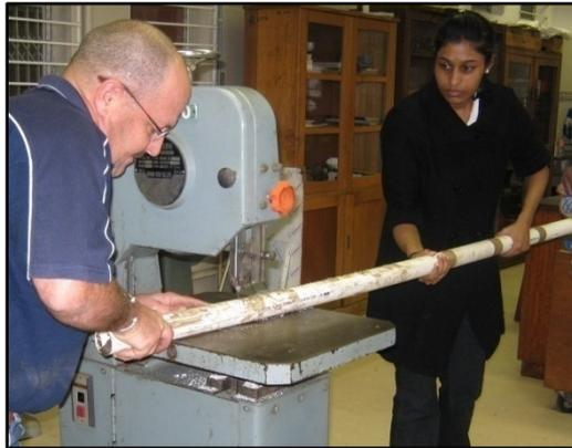
**Figure 31: Careful splitting of the sediment core using an electric saw in the mechanical engineering workshop.**
