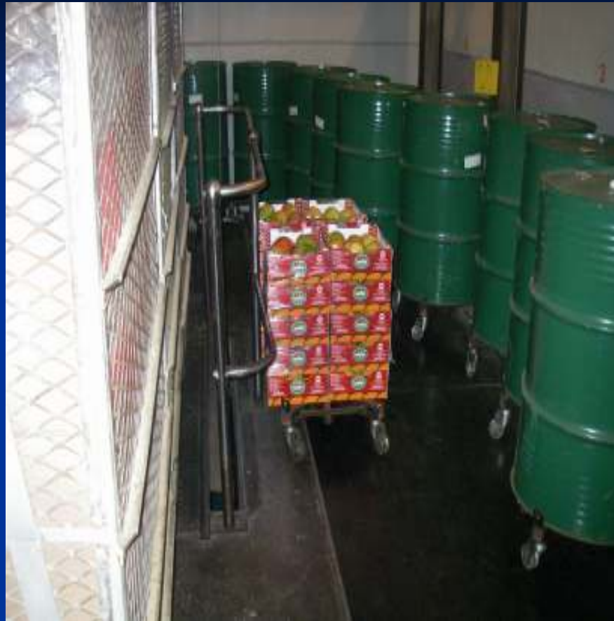
■ Figure 1. Cartons stacked on trolleys facing the gamma radiation source.
