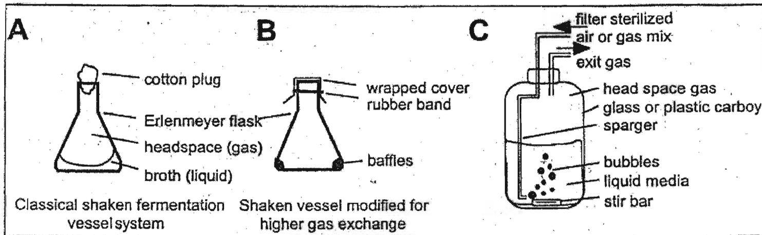
Figure 1.2. Diagrams illustrating common small-scale liquid fermentation systems (Hilton, 1999).
