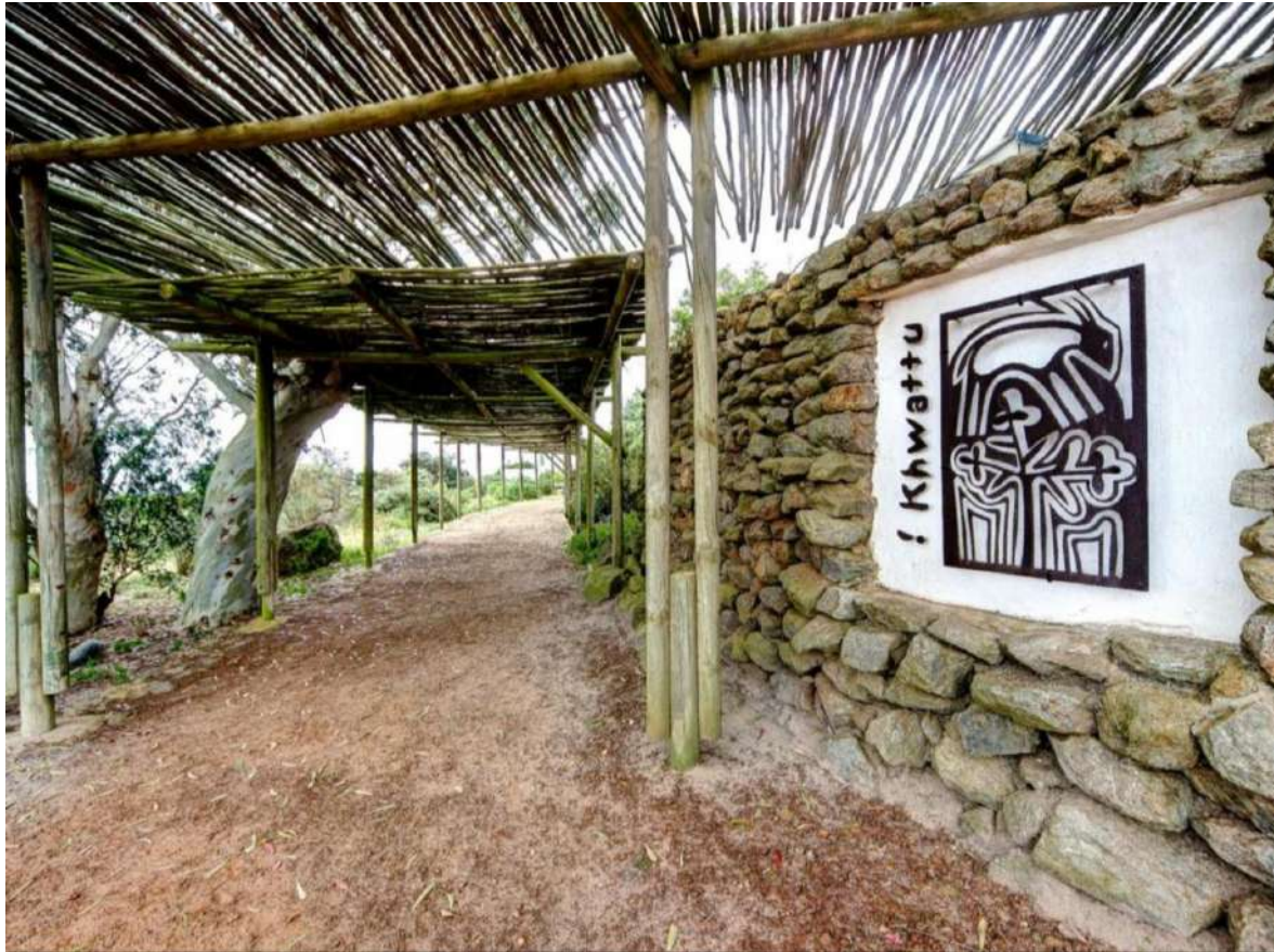
Plate 6.10 Shades and privacy provided by the latte screens made from locally harvested wattle branches (!Khwattu - The "Embassy" of the San - Home to a Very Different Museum, 202)
