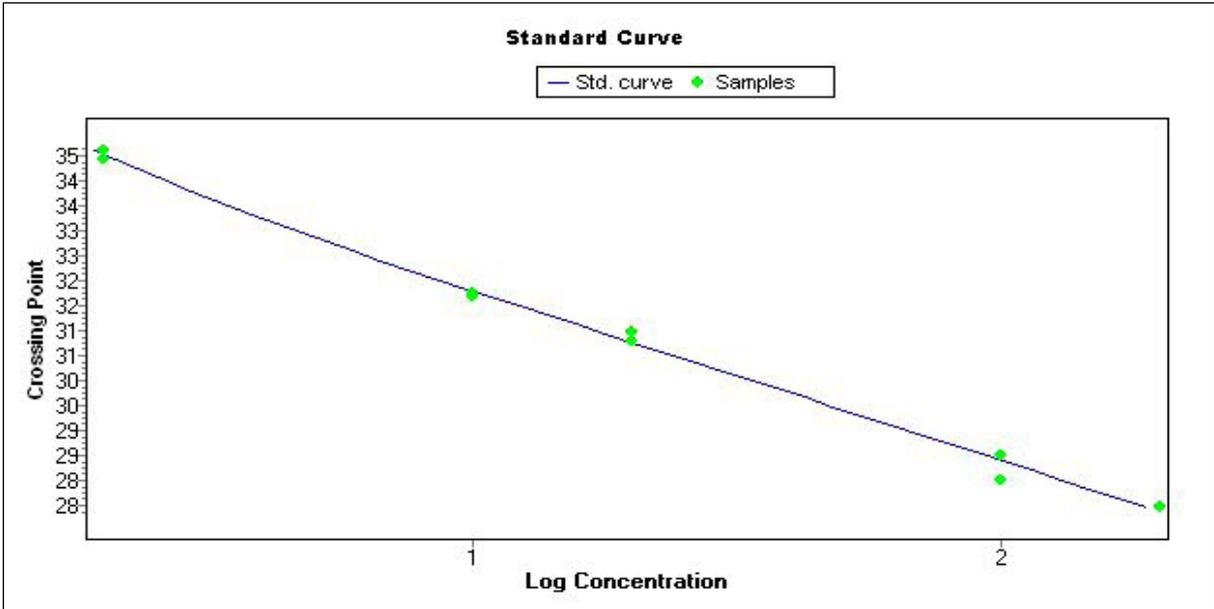
**Figure 28:** The standard curve constructed for GAPDH. The calibration curve shows the crossing points (cycle number) of each standard plotted against the logarithmic concentration.
