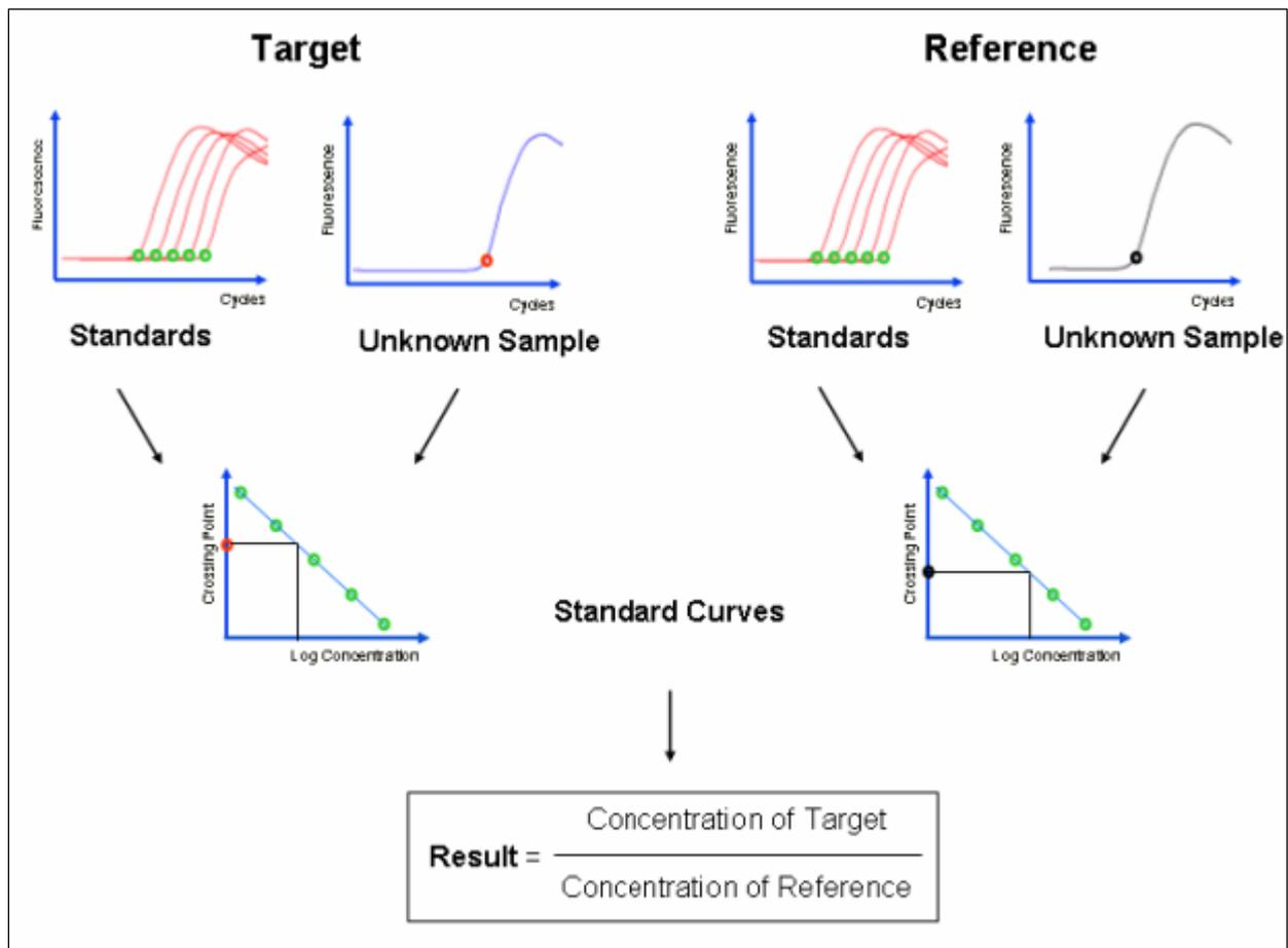
**Figure 11:** Principle of relative quantification (Roche Applied Science Tutorial LightCycler Software 4.05)
