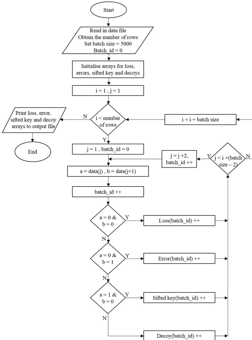
Figure 4.7: The logic flow chart of the sifting programme illustrates how the raw key measured from the system is separated into the sifted key and losses. The errors in the key are counted and this value is used to calculate the QBER. The raw key data was separated into batches of 5000 bits so that the key generation rate and error rate could be calculated per second.
