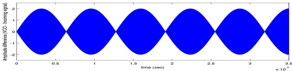
Figure 5.17: A graph showing the amplitude difference between Alice's signal and Bob's VCO signal. In the non-linear case using the parameters listed in Table 5.1, the frequencies of the two signals differed by 15 687 Hz at the beginning of the transmission, hence the signals move in and out of phase with each other at a faster rate compared to the linear case. In this graph, the signals are out of phase by  $\pi$  rad at  $31.8 \mu\text{s}$ .
