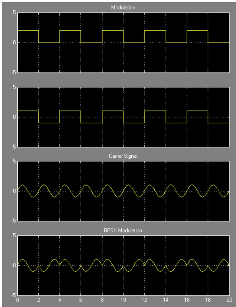
Figure 5.3: The result of the BPSK simulation is shown. a) shows the Modulation signal with an amplitude of 2 V. b) shows the Modulation signal, now shifted by -1 V so that the amplitude is between -1 V and 1 V. c) shows the Carrier signal and d) shows the product of the Carrier signal and the shifted Modulation signal. A phase change occurs every 2 seconds, representing a change in the bit value of the Modulation signal.
