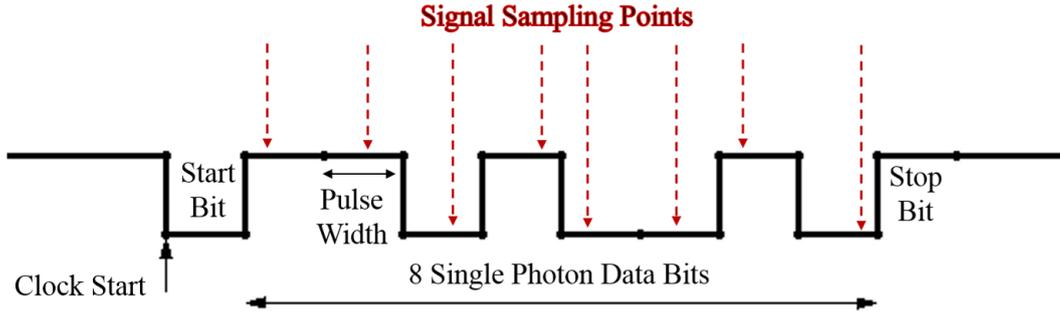
Figure 5.1: A figure showing the signal structure of asynchronous transmission. Asynchronous transmission begins with a Start bit which serves as the synchronisation indicator. The pulse width of each bit is agreed upon before the transmission begins and the receiver is able to measure the 8 data bits following the Start bit. The Stop bit indicates that the data has stopped, pending the transmission of another Start bit.
