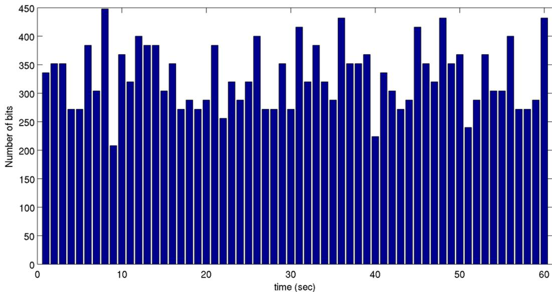
Figure 4.3: A plot of the raw key generation rate per second, measured over one minute.
