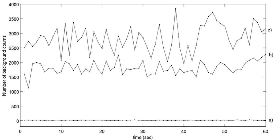
Figure 4.5: A graph showing the measurements of background noise for different lighting conditions in the laboratory. Graph a) shows the detector dark count rate, measured in a dark room. Graph b) shows the background noise measured with dim laboratory lights on. Graph c) shows the background noise with fluorescent laboratory lights on.
