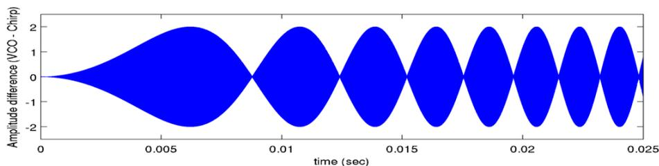
Figure 5.8: A graph showing the difference in amplitude between Alice's signal and Bob's VCO signal. As Alice's signal increased in frequency due to Doppler shift, the two signals moved in and out of phase with each other. Points of maximum amplitude on this graph indicates when the signals were out of phase by  $\pi$ rad. Points of zero amplitude on this graph indicate when the signals were in phase.
