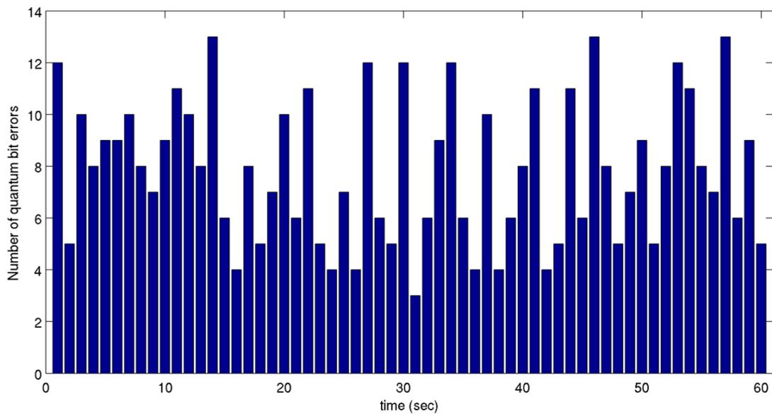
Figure 4.6: A graph showing the total errors per second identified in the sifted key for a duration of one minute. The errors represent dark counts and noise in the system.
