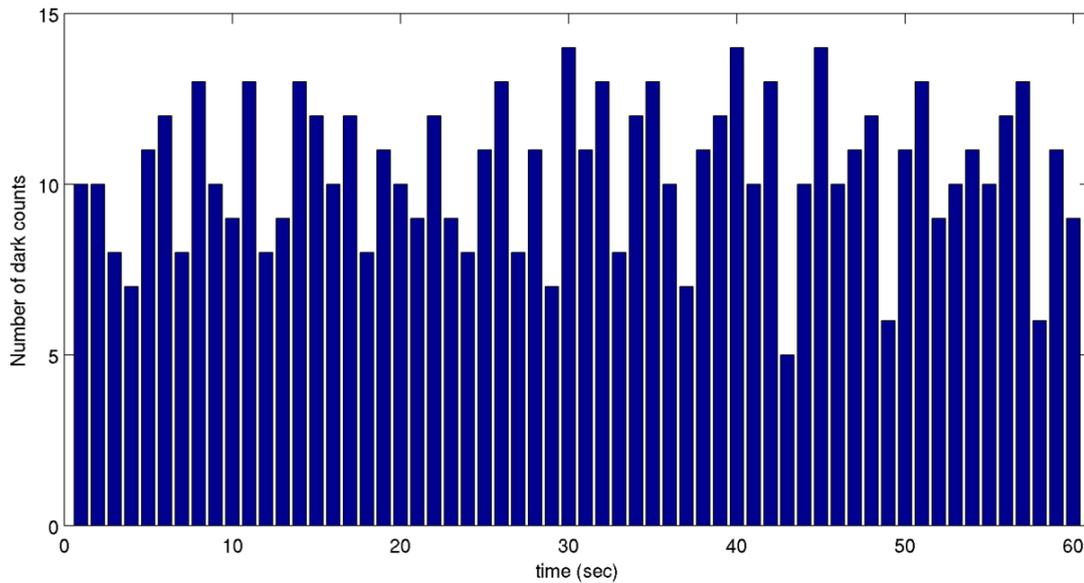
Figure 4.4: A plot of the dark count rate per second, measured over one minute for the single photon detector in Bob's detection line.
