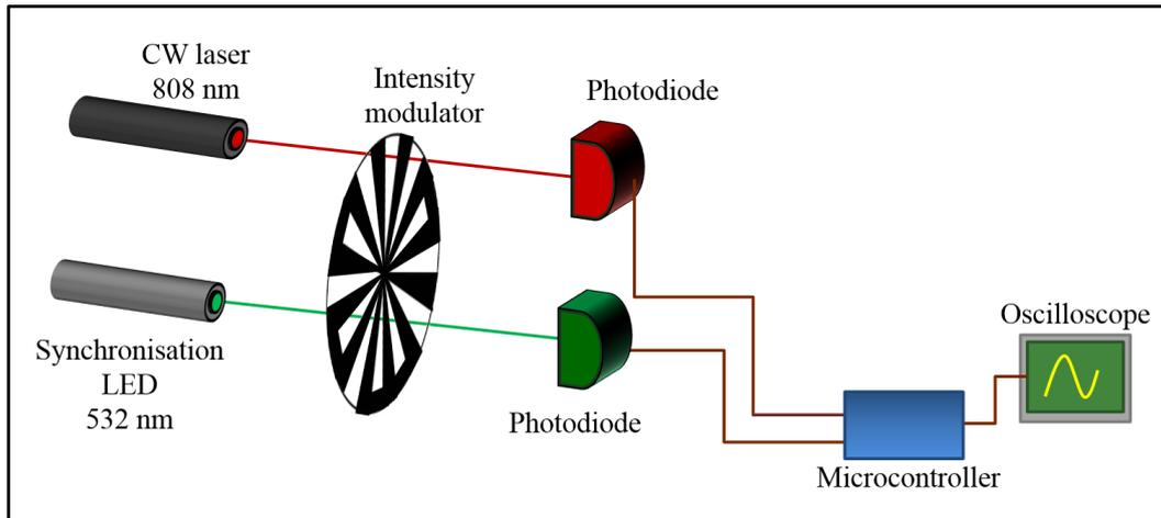
Figure 3.10: A temporary photodiode was added into the system to precisely align the relative positions of the 808 nm laser and the green LED. The signals from both photodiodes were measured by the microcontroller and displayed on an oscilloscope.
