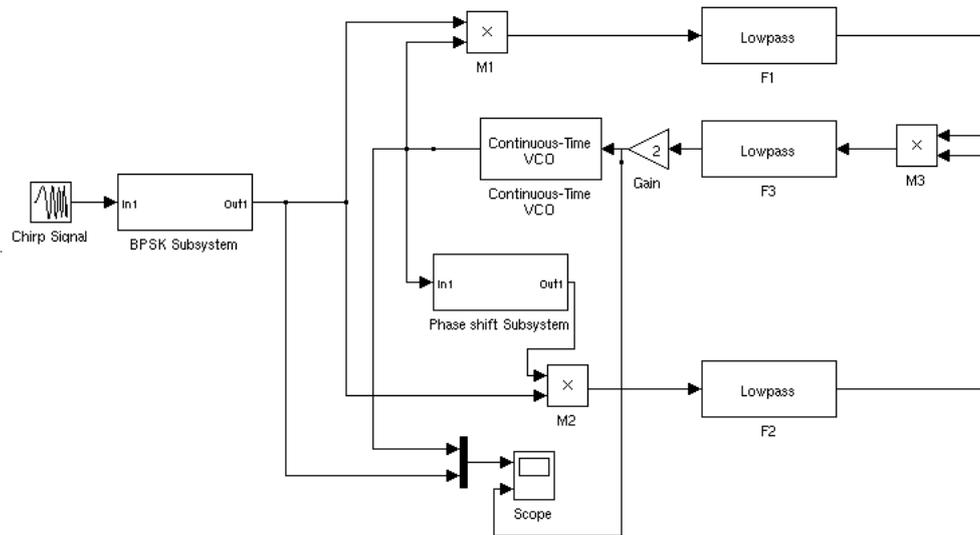
Figure 5.12: A figure showing the simulation setup for the Costas loop, with a BPSK modulated signal with a linearly changing frequency from Alice. The parameters for the VCO were set to those of a commercially available VCO. Since the input of the VCO needed to be of the order of 0.5 V to 1 V, the signal required amplification. The scope indicates the points from which the output results were viewed. The results are shown in Figure 5.13.
