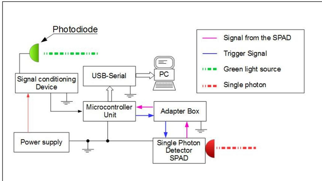
Figure 3.12: A block scheme of the electronic connections used to synchronise Alice's module with Bob's detectors. The components shown in this diagram were all housed in Bob's unit. The photodiode which measured the green LED transmitted its signal to the microcontroller which then triggered the detectors via the connection panel on the adapter box.
