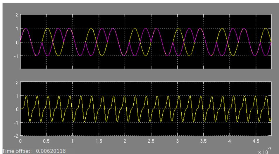
Figure 5.13: The simulation result showing the extraction of the carrier signal from a BPSK modulated signal with a linearly changing frequency. a) shows the comparison of Alice's BPSK modulated signal, shown in pink, with Bob's VCO signal, shown in yellow. The sinusoidal VCO signal was able to match the changing frequency of the BPSK modulated signal, thus synchronising the two modules. The amplified input to the VCO is shown in b).
