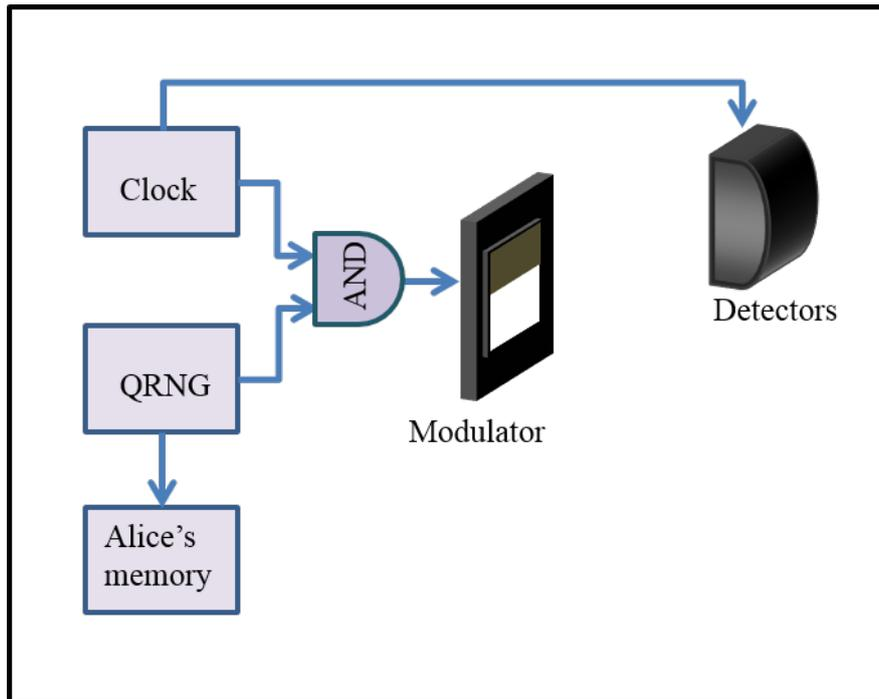
Figure 3.3: The clock rate in Alice's system must be combined with the bit string of the quantum random number generator with a logical AND gate in order to control the pulse modulator. The clock rate is also transmitted to Bob in order to synchronise the Bob's detector gate with the arrival time of a pulse. The bit string of the QRNG must be stored in Alice's memory for use during post processing.
