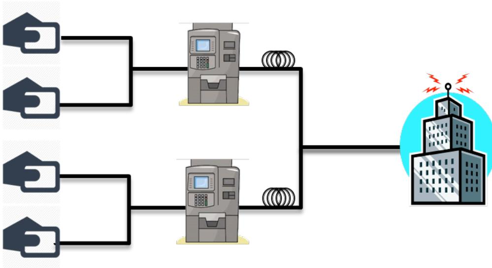
Figure 2.5: A diagram showing an example of a star topology network used to connect individual QKD devices to a central central node [4]. Multiple users are able to exchange a key with an intermediary station (node) such as an ATM. This station in turn, performs a QKD exchange with a central node such as the central office of the company. A secret key is established between the user and the vendor through the process of node hopping.
