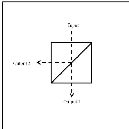
Figure 3.4: A beam splitter is able to separate incoming light into two paths. The first output is transmitted through the prisms and the second output is reflected orthogonally at the boundary between the two joined prisms.
