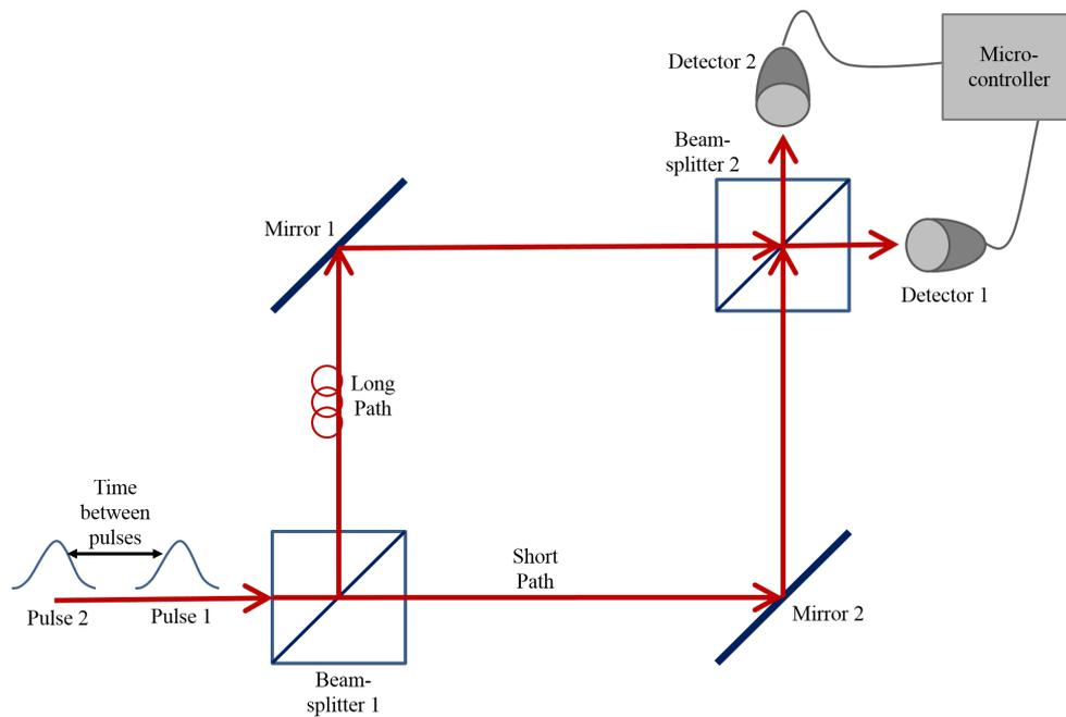
Figure 3.5: A diagram of a Mach-Zehnder interferometer which forms the monitoring line of Bob's module. The incoming pulses are randomly separated at Beam-splitter 1, choosing between the short or long path of the interferometer. Any pulses propagated through the long path will undergo a delay which will displace them by one time bin. The pulses are incident on Beam-splitter 2 and the photons are measured by Detector 1 or 2. Both detectors are triggered by the Microcontroller.
