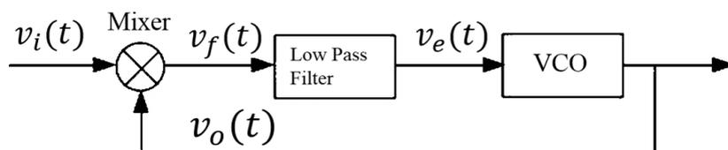
Figure 5.4: A schematic diagram of a PLL. The VCO signal is combined with the incoming signal  $v_i$ . The resulting signal is filtered so that only low frequency terms remain. The filtered signal is used to adjust the VCO, providing a continuous feedback loop.
