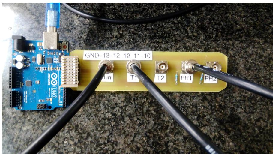
Figure 3.13: A photo of the panel of coaxial connections on the adapter box which linked the green LED, trigger signal and detector signal to the microcontroller.
