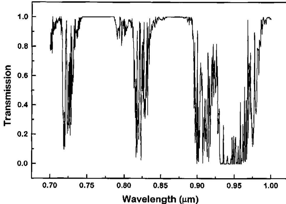
Figure 3.1: A graph showing windows of optimal transmission of different wavelengths in the atmosphere. This image is sourced from [6]
