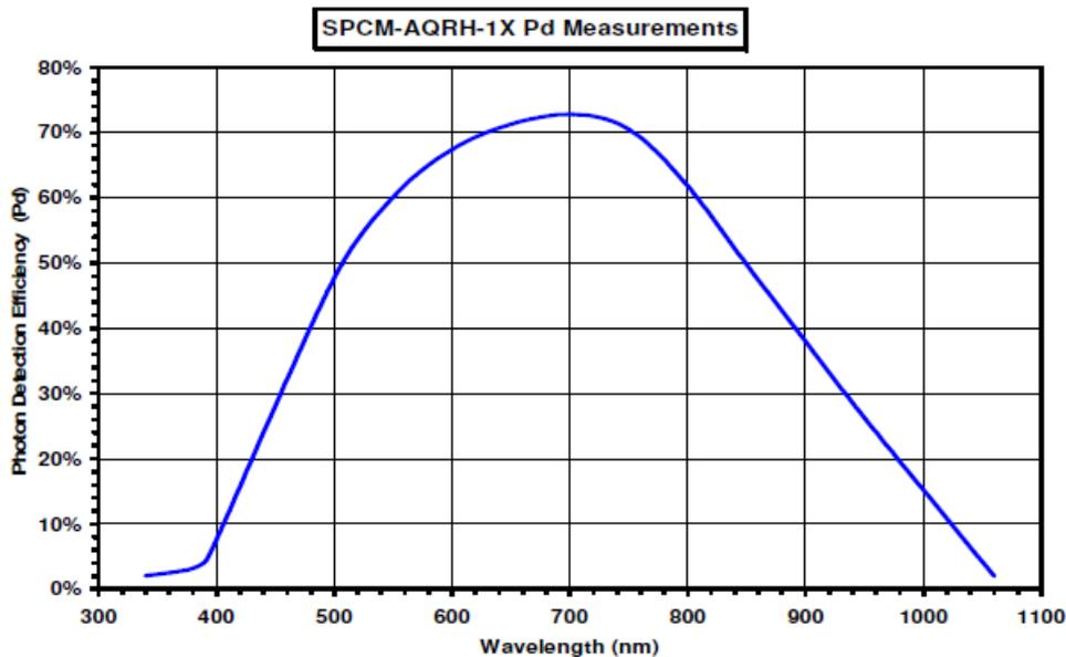
Figure 4.2: A figure showing the detection efficiency of the single photon detector with respect to operating wavelength. For the 808 nm laser used for this system, the detection efficiency was 60%. This image is sourced from [9].
