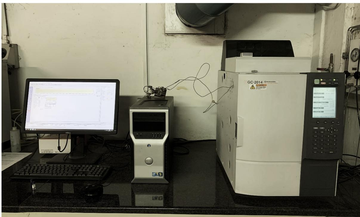
Figure A-4. Image of Shimadzu GC-2014 with PFDP and FID.
