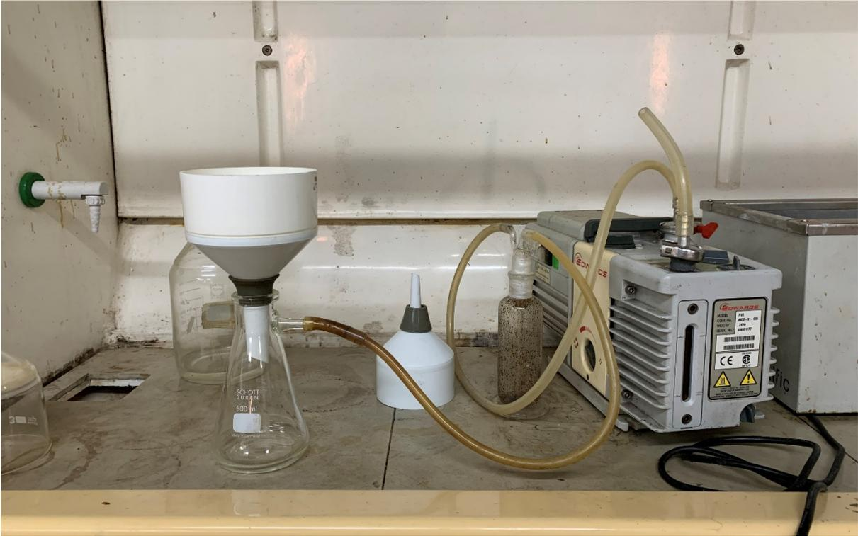
Figure A-5. Image of filtration system with an Edwards RV3 vacuum pump.
