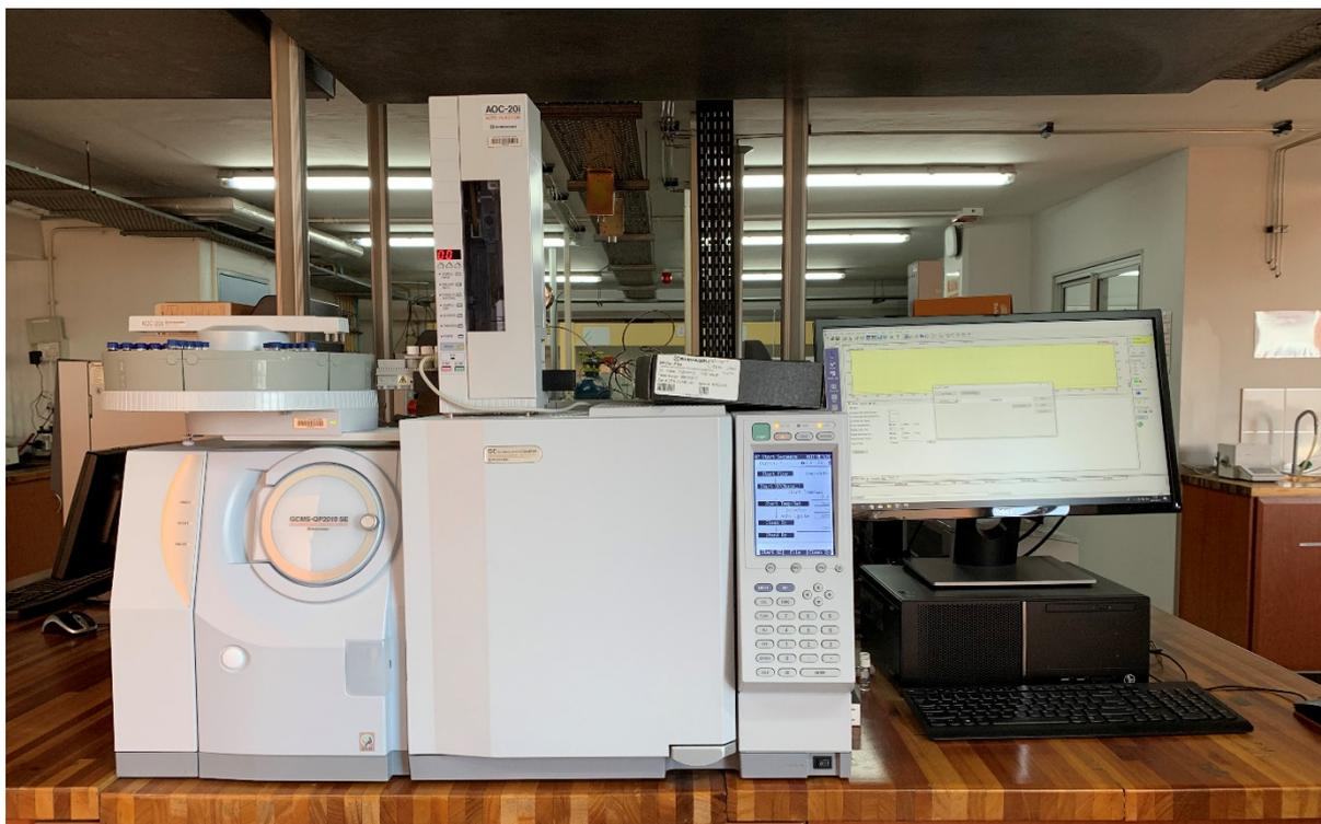
Figure A-3. Image of GC-MS – QP2010 SE Equipped with an AOC-20i auto injector.
