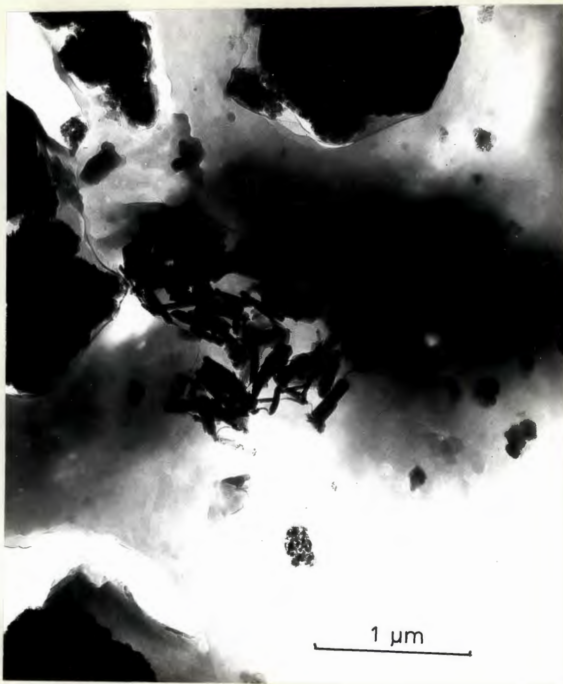
PLATE 6. Electron micrograph of natural clay ( < 2 \mu\text{m} ) from sample no. 6 (X 40 000)
