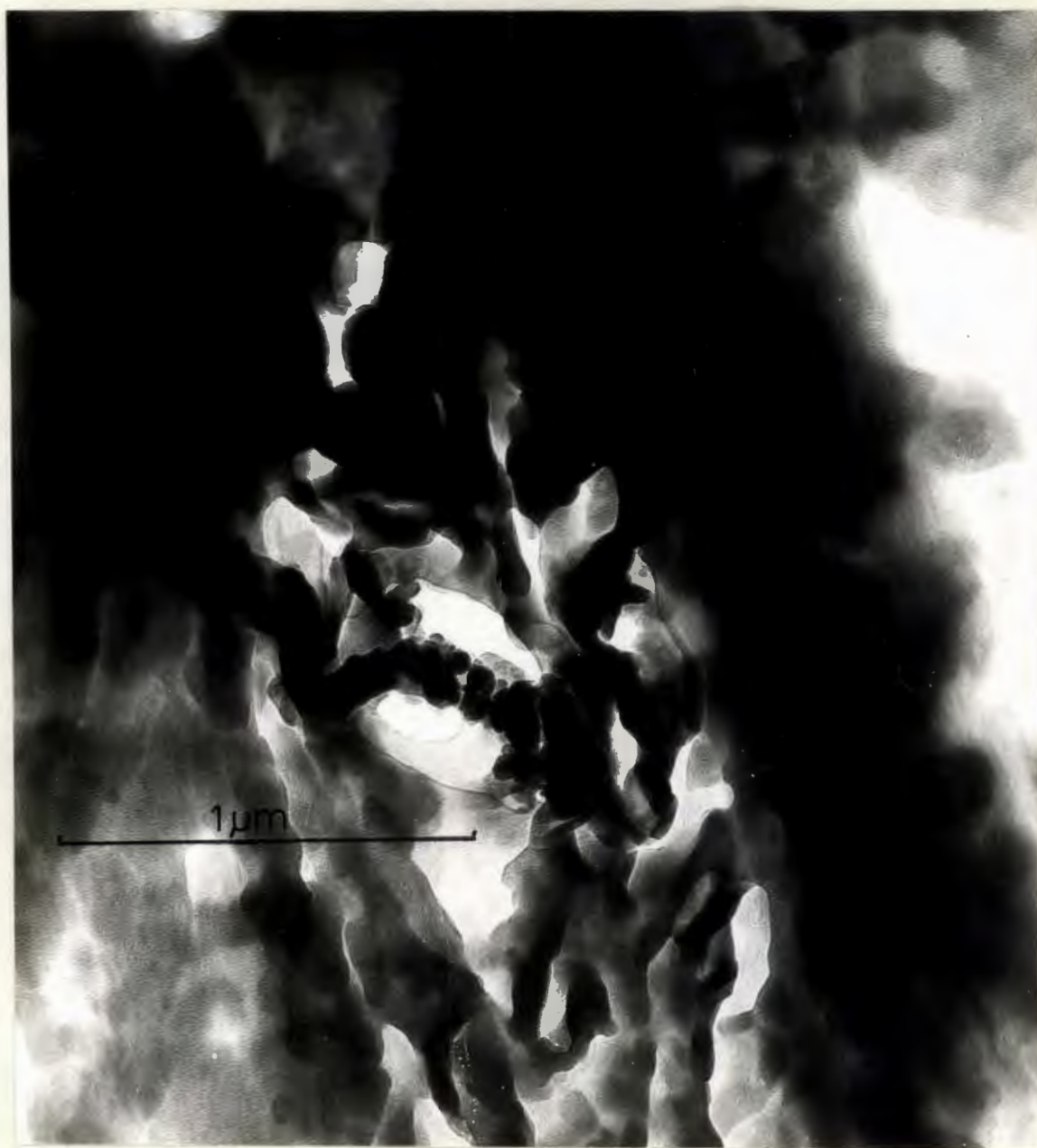
PLATE 7. Electron micrograph of deferrated clay ( < 2 \mu\text{m} ) from sample no. 11 (X 60 000)
