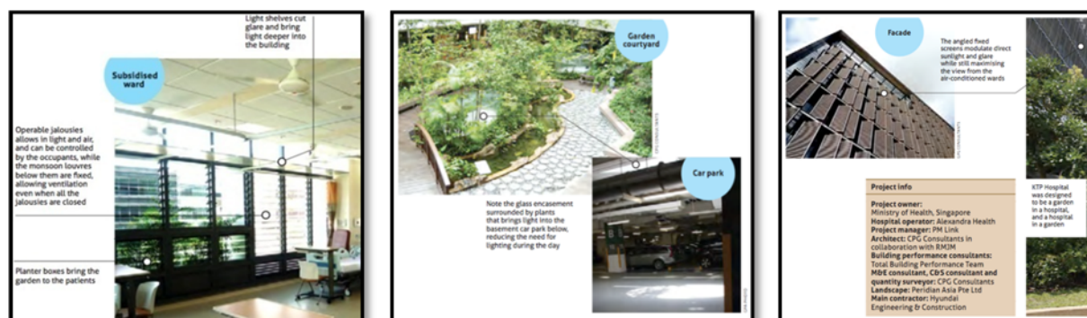
Figure 3.30, 3.31 & 3.32: Window design strategies allow for natural airflow and reduces glare, providing clear storey lighting into basement parking below, angled screens controlling sunlight (www.greenprospectasia.com)
