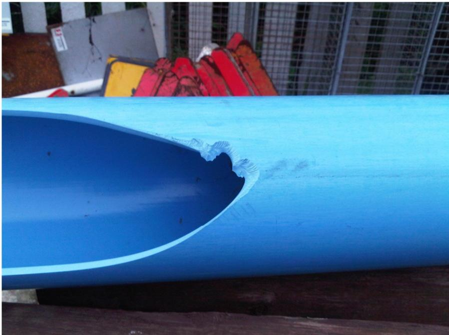
*Figure D.2: Pressure burst on a mPVC main*
