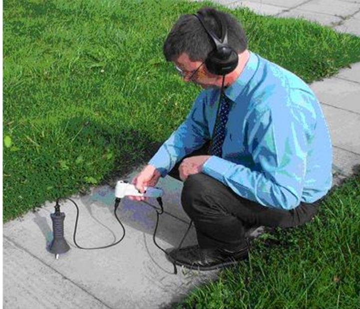
*Figure 3.17: Leak detection using a ground microphone. (Photo courtesy of Mr Chris Otto, 2010)*
