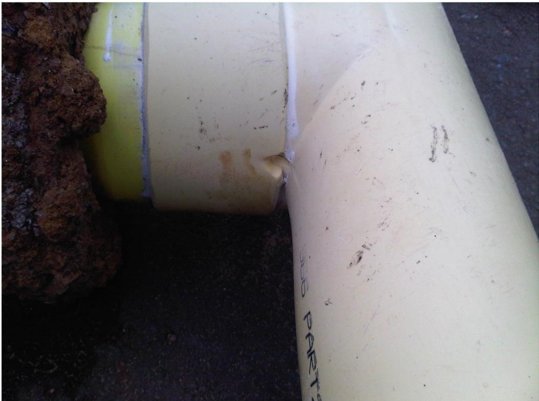
*Figure D.4: Pin hole failure on a PVC tee*
