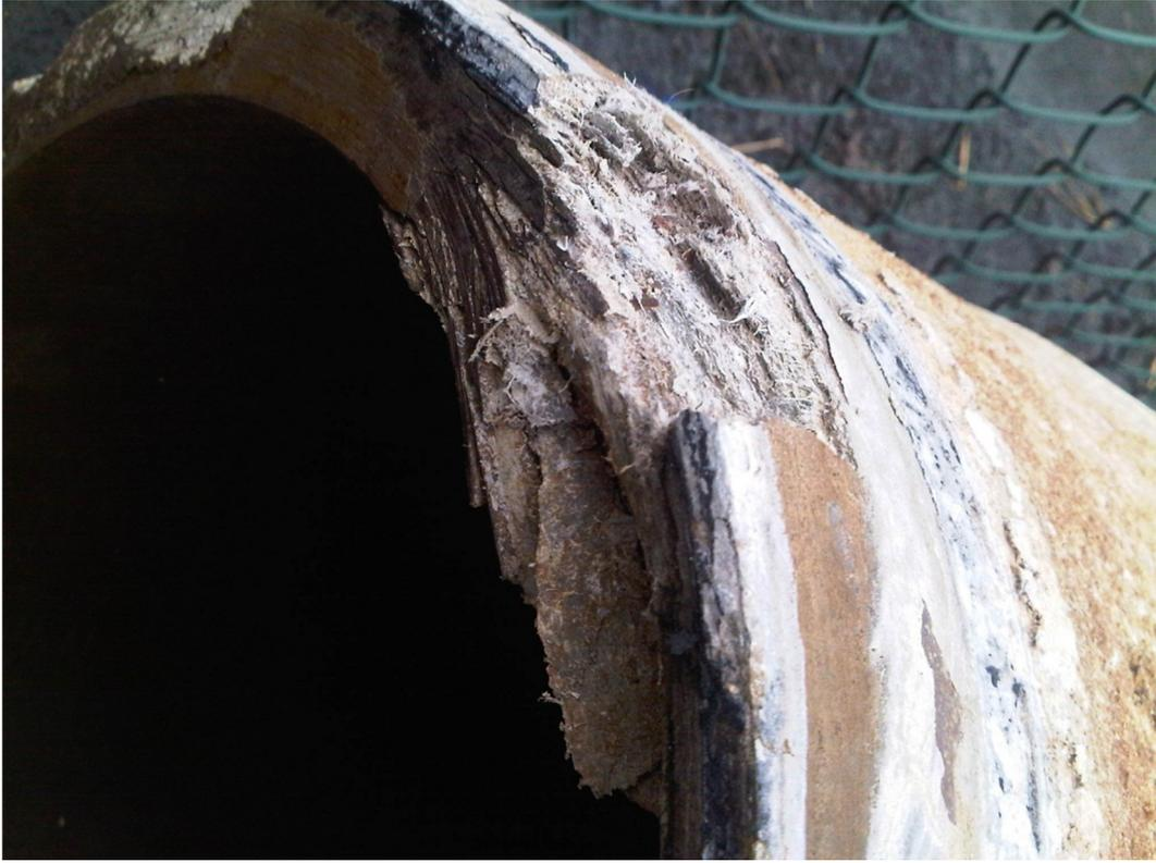
*Figure D.9 AC pipe degraded through soft water attack*
