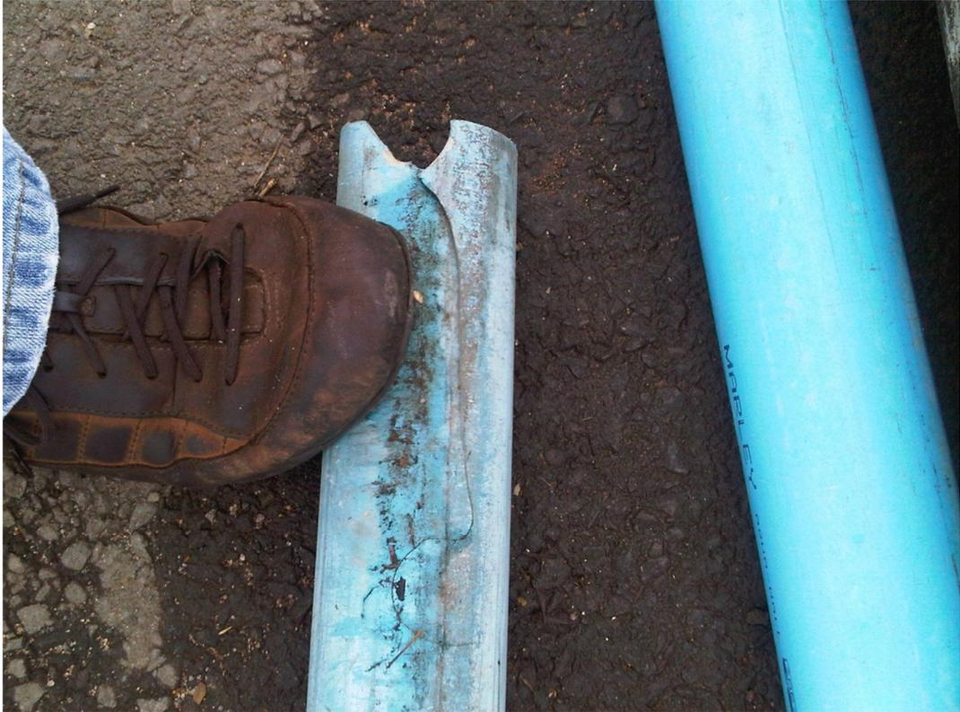
*Figure D.3: Longitudinal Pressure burst on an mPVC pipe*
