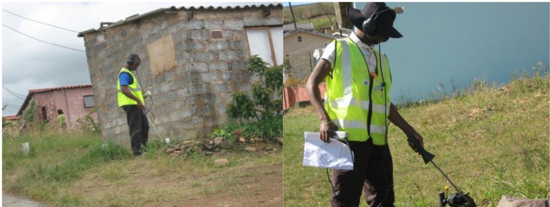
*Figure 3.16: Mechanical Leak Detection using amplified listening stick. (Photo courtesy of Mr Chris Otto, 2010)*
