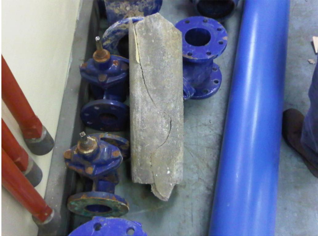
*Figure D.5: Longitudinal pressure burst on an AC pipe*
