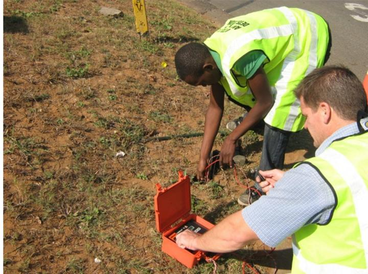
Figure 3.19: Leak Detection Using Leak Noise Loggers. (Photo courtesy of Mr Chris Otto, 2010)
