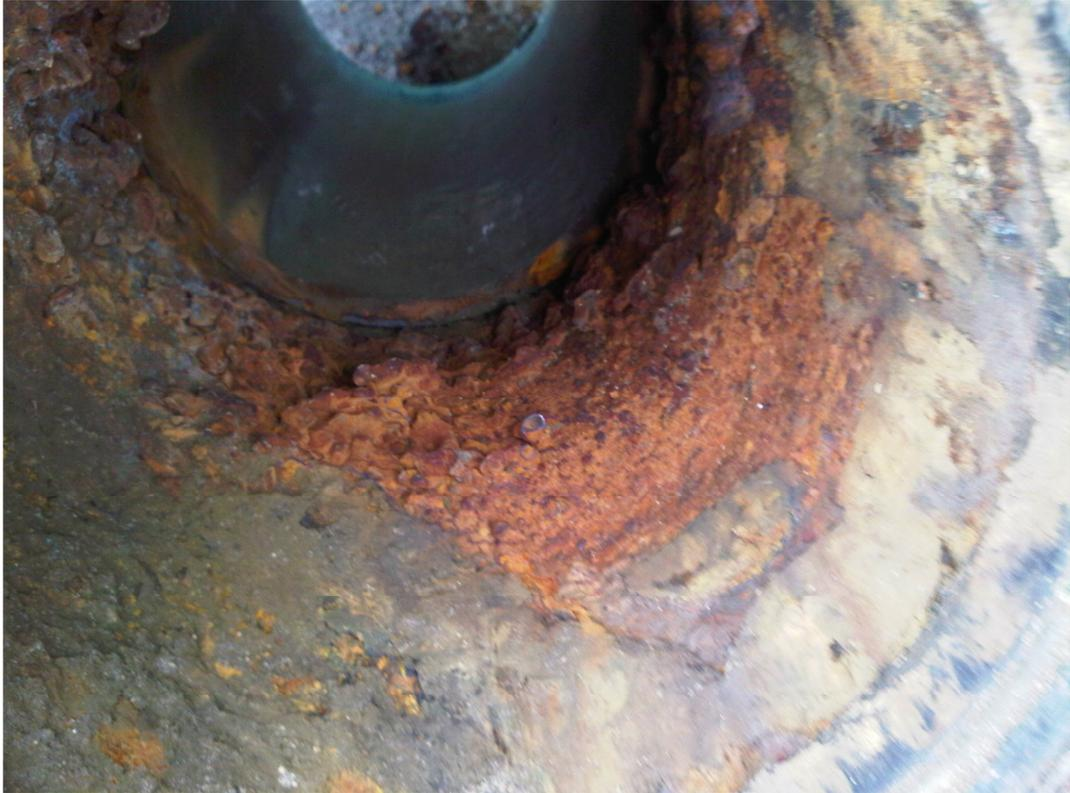
*Figure D.11: Pipe tuberculation in an unlined cast iron pipe*
