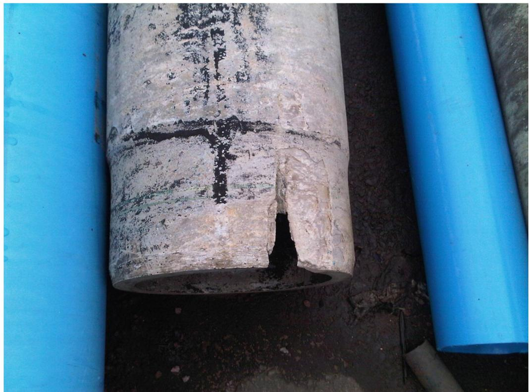
*Figure D.8: AC pipe collar failure*
