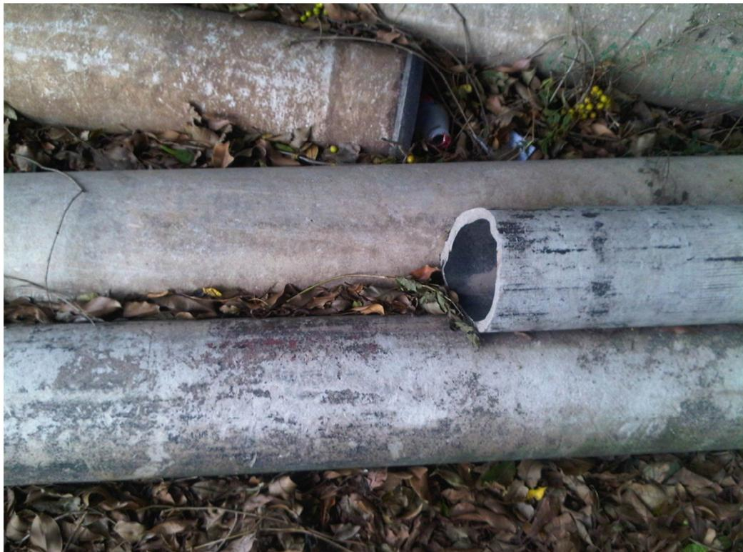
*Figure D.6: Ring fracture on an AC pipe caused by settlement*
