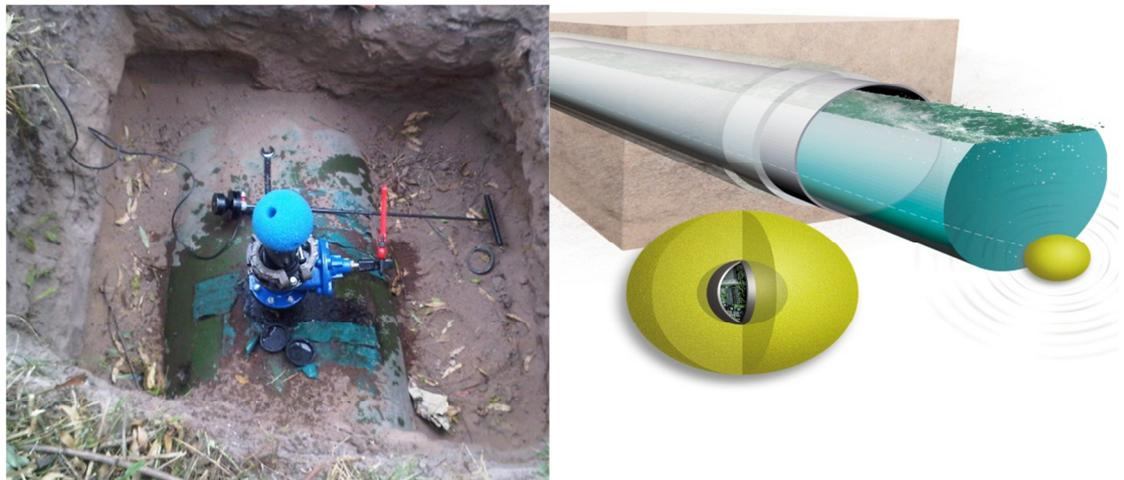
Figure 3.24: Smart Ball Internal Noise/Leak Technology (SSIS Consulting Engineers, 2010)
