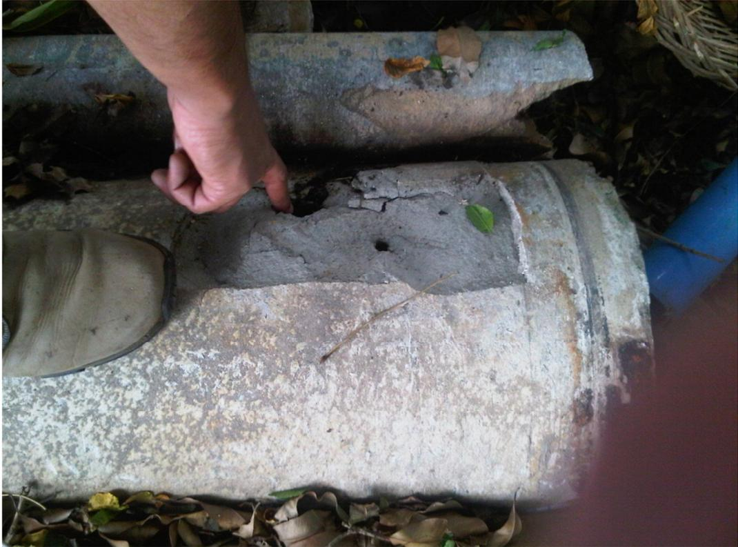
*Figure D.7: Hole failure in an AC pipe*
