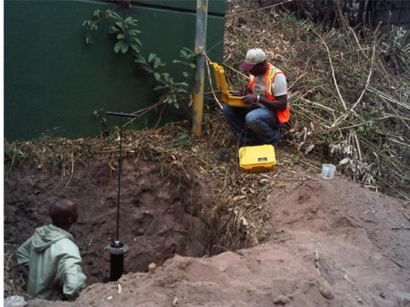
*Figure 3.25: Smartball Leak Detection (SSIS Consulting Engineers, 2010)*
