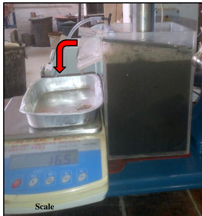
Figure 3-2: Collection of concentrate without the use of scraping the froth into the collection container. In this particular case, the longer nearly horizontal baffle was used.
