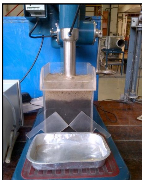
Figure 4-4: Flotation test with the use of scraping paddles. Two paddles were used to scrape off the surface of the froth in constant intervals of 15 seconds according to laboratory flotation standards.
