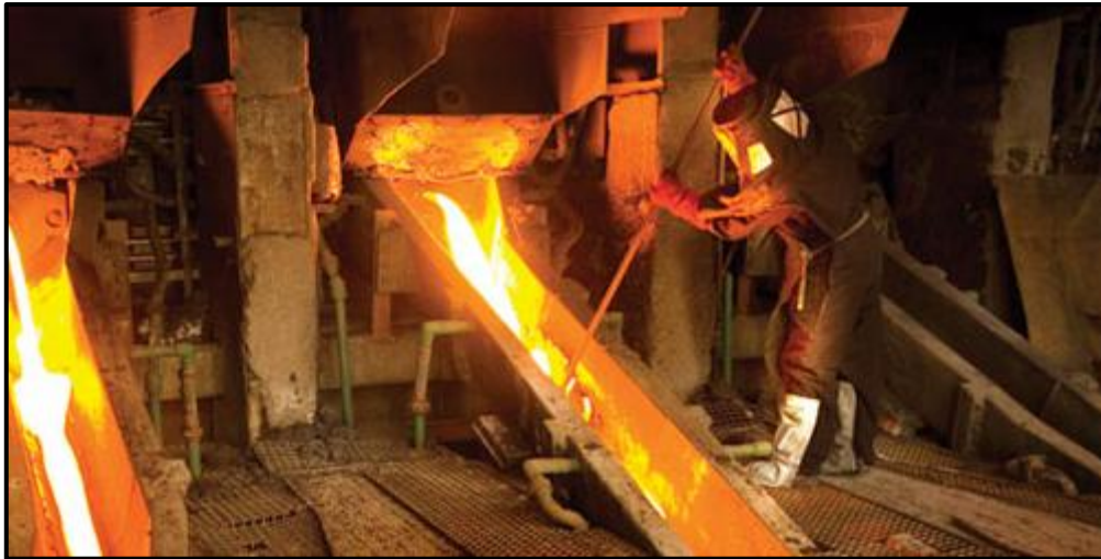
Figure 2-9: Exit of smelter containing the PGM + Au and Ni–Cu matte. The matte then goes for further refining to separate precious metals from base metals. The base metals are removed by standard electrolyte techniques (Anglo American, 2008).
