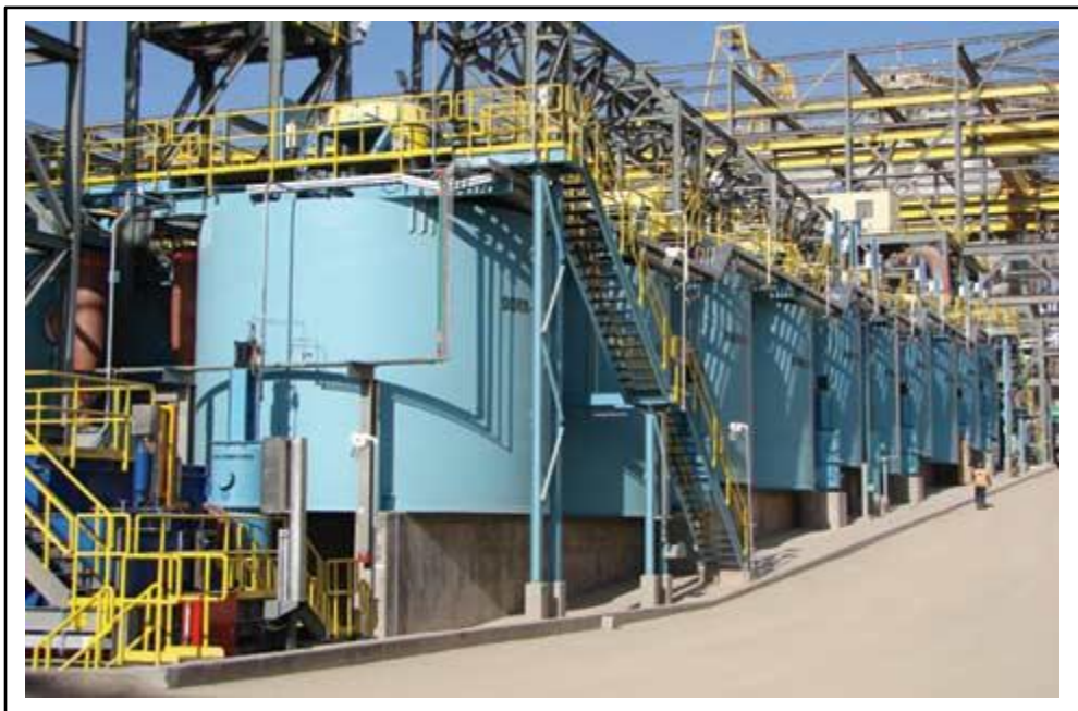
Figure 2-17: Bank of WEMCO® SmartCell™ flotation cells in a flotation circuit (taken from FLSmidth, 2010).
