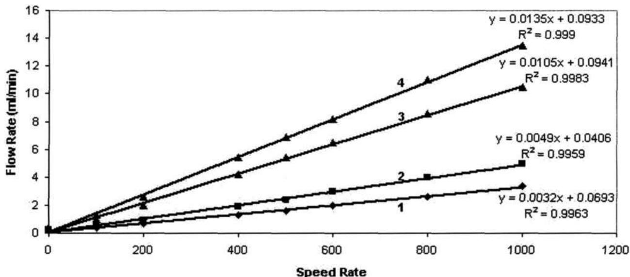
Figure 6.5: Flow Rate versus Pump Speed
