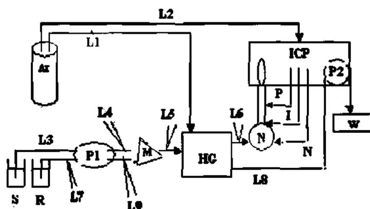
Figure 6.2: Schematic Diagram for HG-ICP-AES Set-Up
