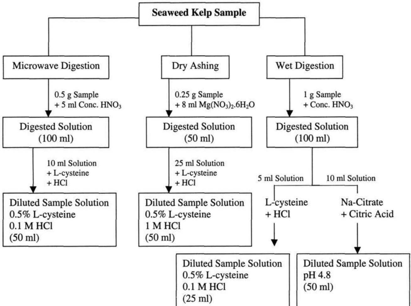
Figure 6.3: Flowchart for Sample Digestion Procedure
