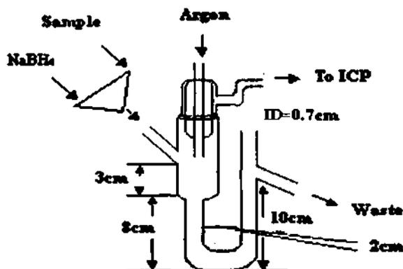
Figure 6.1: Gas Liquid Separator Apparatus
