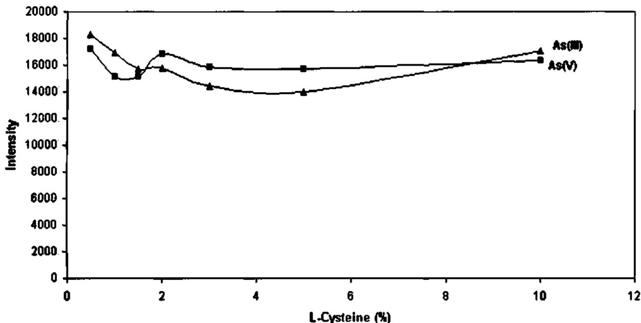
Figure 6.7: Effect of L-Cysteine on the Responses of As(III) and As(V)
